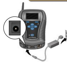
1 Plug the AC adapter supplied with the *StarMOBILE* kit into the DC power connection of the *StarMOBILE* and the AC power cord into a suitable wall outlet.
