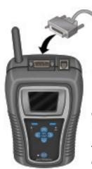
Press vehicle cable connector firmly into jack.
