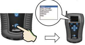
4 Press the Power button on the *StarMOBILE* device. Within 20 seconds, the LCD screen should display the initial screen.
