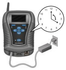
3 Allow the *StarMOBILE* system to charge for at least four hours. The rate at which the LED blinks should reduce in frequency. However, since the system will continue to charge, the LED may occasionally blink *red*.
