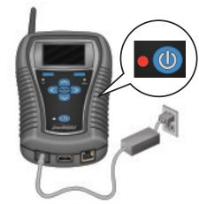
With the StarMOBILE device powered off, observe that the power LED of the StarMOBILE system is blinking red. This indicates that the battery is charging.
