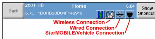
The icon furthest to the right displays StarMOBILE device and vehicle connection information. When the StarMOBILE Desktop Client is not connected to a StarMOBILE device, the SM icon is shown with a red slash. Clicking on the icon in this state will launch the discovery wizard which allows the StarMOBILE Desktop Client pc application to connect to a SM device (if one is available on the network).
