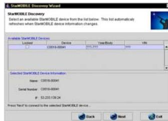
This is the normal behavior, and does not indicate a problem. The reason the question marks are displayed is because the StarMOBILE is expecting there to be a Central Gateway ECU that it can retrieve the Year, Body and VIN information from. The 2006 KJ does not have a Central Gateway ECU so the tool returns '???'.
