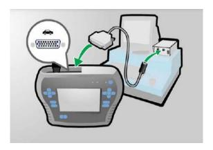
Note: You can optionally connect your StarSCAN tool to a vehicle using your StarSCAN vehicle cable, but make sure the vehicle's battery has a full charge or problems may result when updating your StarSCAN software.
